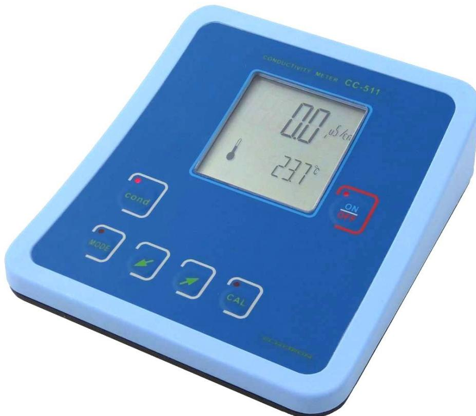
The set includes **CT2B-121** temperature probe with **Pt-1000B** resistor and accurate **ECF-1** conductivity cell. Measuring range: 0 ÷ 400 mS/cm is sufficient for conductivity measurements in majority of liquids of maximal concentration, e.g. aqueous soil extracts and water with grease or oil. Metal electrodes are easy to clean. Plastic housing protects from mechanical damage.
